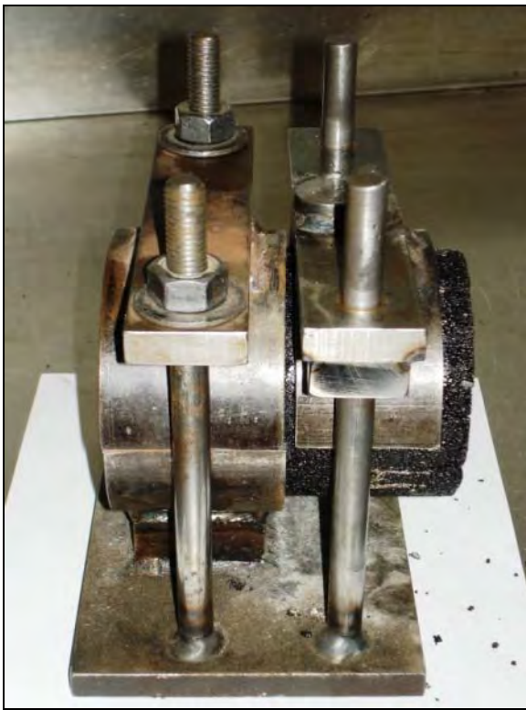
Figure 3. Mounted Specimen and Shear Plane
